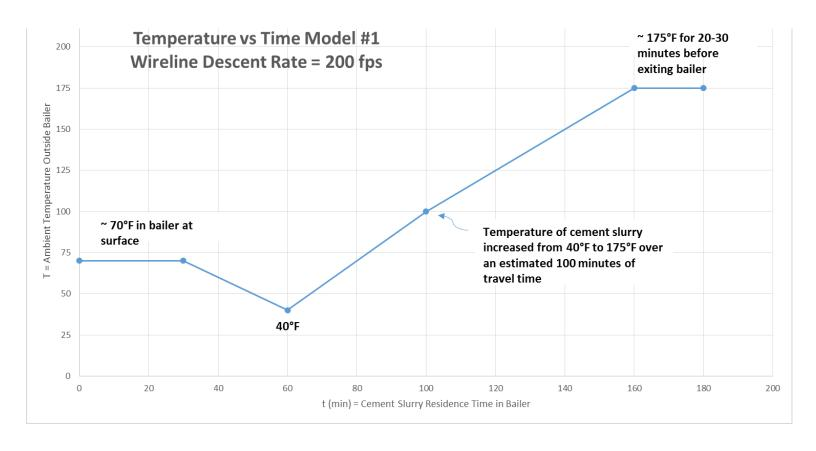
Figure #1: \_\_\_\_\_ Test of Temperature vs Time
